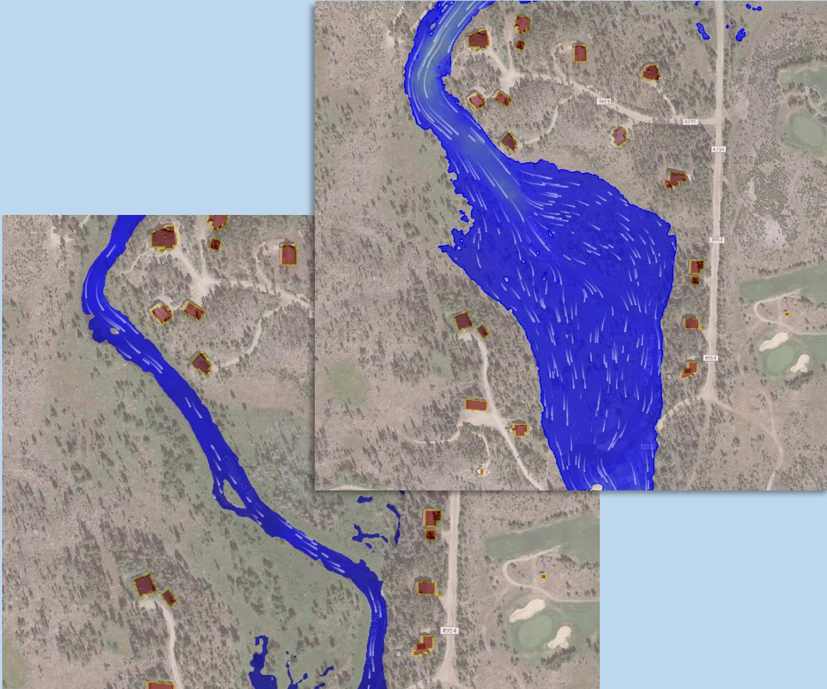
Pre (left) and post (right) fire flood hazard mapping within the East Troublesome burn perimeter.
