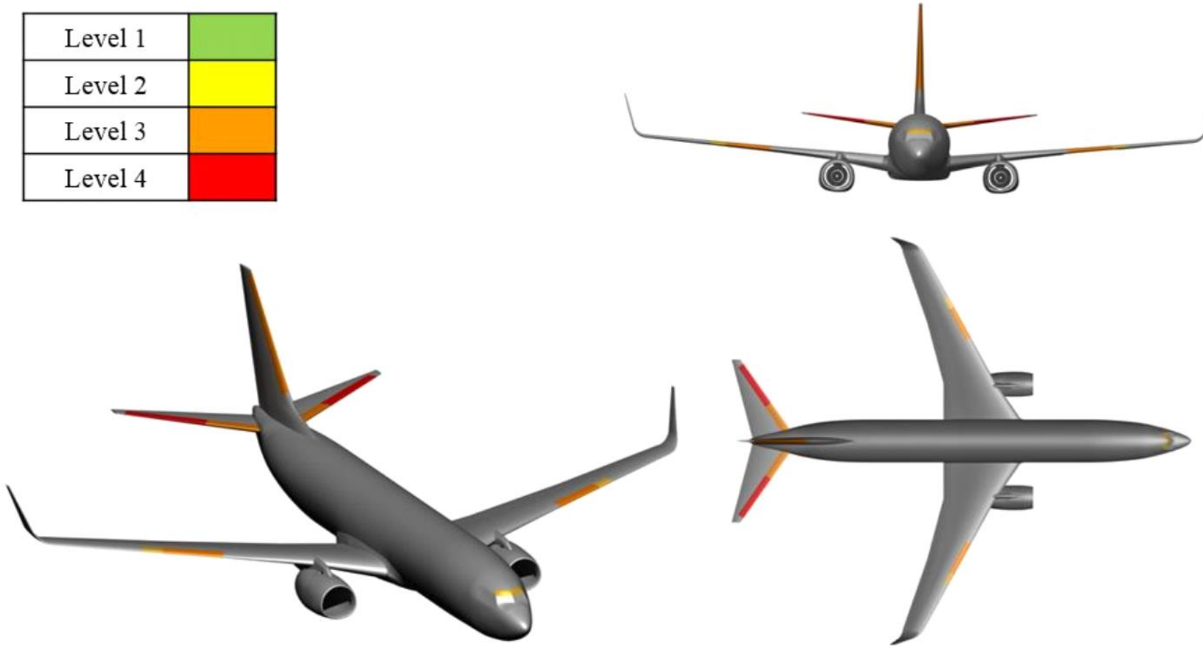
Figure 240. Summary of collision severity levels on commercial transport jet
